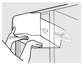
2 Lift and pull forward again to remove the bin.
